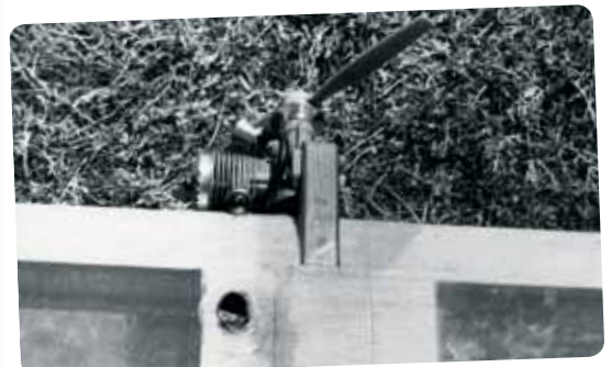
Note the exhaust pipe mount. You might think it burned the wing but it worked which allowed rear exhaust port engines to be used.
