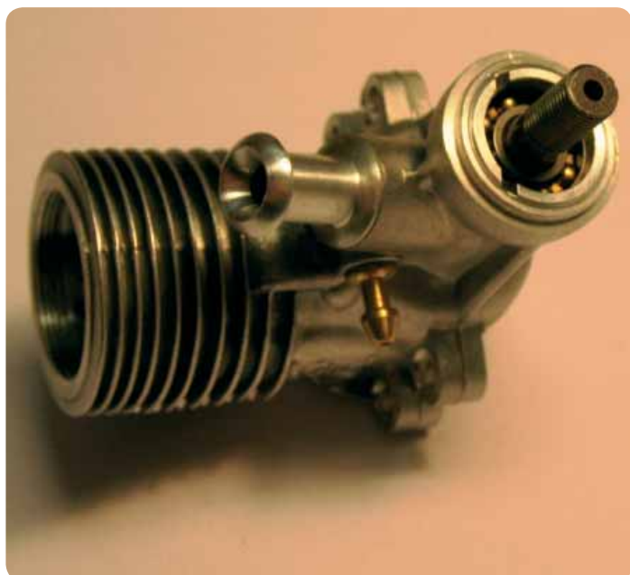
The front bearing is locked with an aluminium ring..
