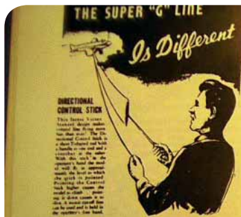
Fig. 7. New approach by Victor Stanzel with Tee stick control plus engine control from third line.
