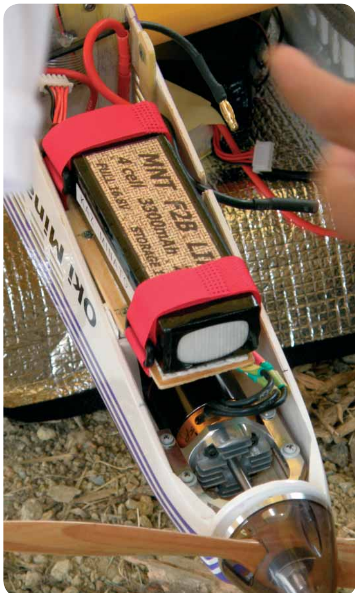
Oki Minatos (Japan) elmotor-installation.
