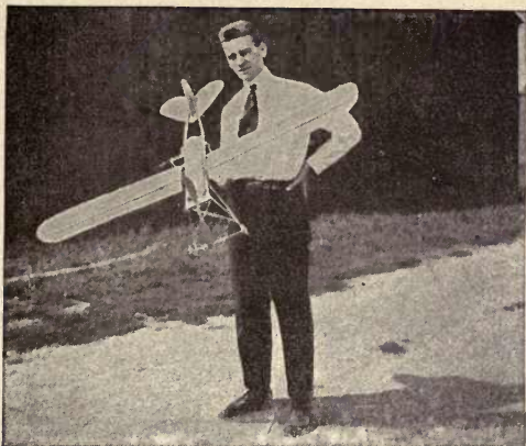
John McMahon and his compressed air driven monoplane
