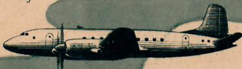
HANDLEY PAGE HERMES 5 — 4 Theseus Propeller Turbines
