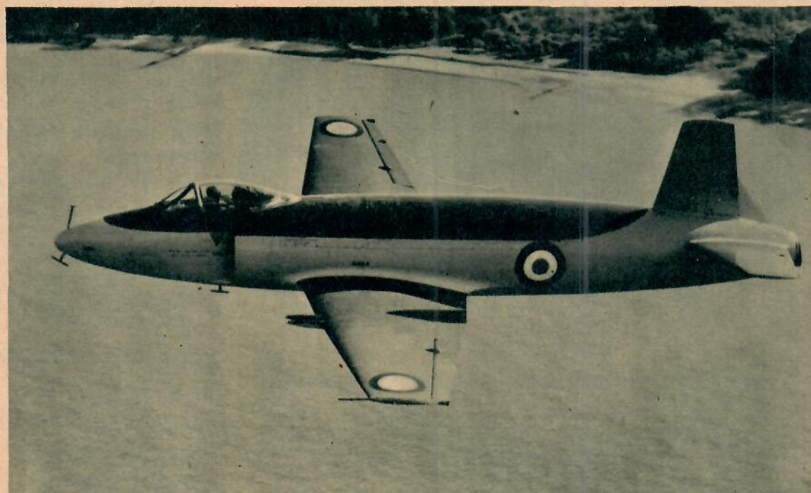
VICKERS SUPERMARINE "ATTACKER" MARINJAKTPLAN utrustat med Rolls-Royce "Nene" reamotor
